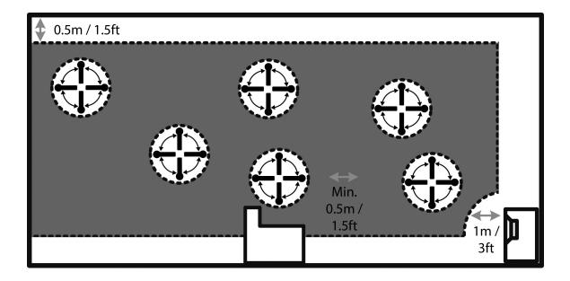
The microphone should not be closer than 0.5m/1.5ft from the floor, ceiling, and walls. The microphone should be at least 1m/3ft from the front of the loudspeakers.
