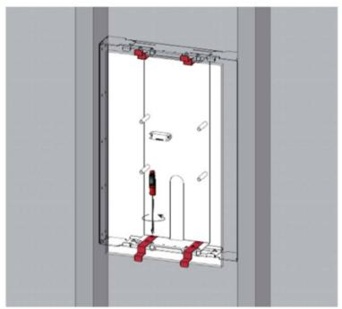
Connect the speaker cable to the speaker in accordance with the connection label on the back of the speaker. Place the speaker in the wall.
