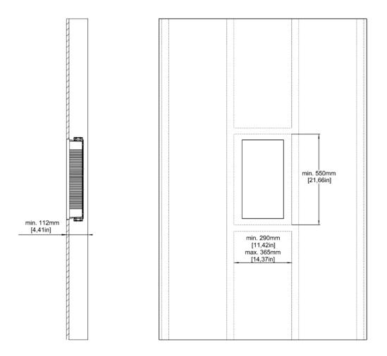
Note: The total combined weight of a Model M speaker and frame is 15 kg/33 lbs. Screws and ceiling must be able to carry this weight.
