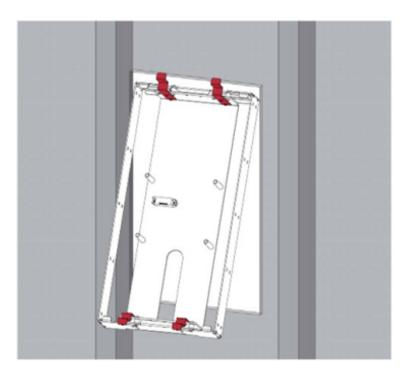
When positioning the wall brackets, make sure that the red brackets are spaced so their distance to the sides of the cutout are exactly the same.
