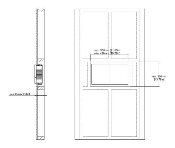
Note: The total combined weight of a Model M speaker and frame is 15kg/33lbs. Screws and wall must be able to handle this weight.
