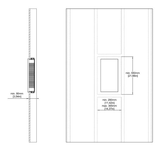
Note: The total combined weight of a Model M speaker and frame is 15kg/33lbs. Screws and ceiling must be able to carry this weight.
