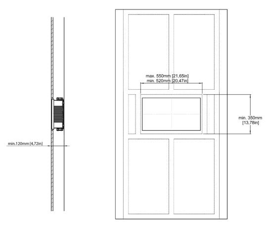
Note: The total combined weight of a Model M speaker and frame is 15kg/33lbs. Screws and wall must be able to handle this weight.
