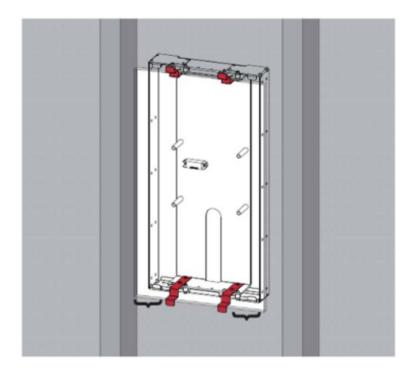
Push the adjustable frame sides all the way out so they touch the inside studs.
