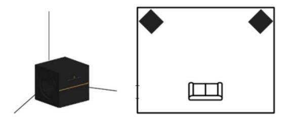
If a corner placement isn't possible, the Boundary Woofers should be placed up against the wall.
