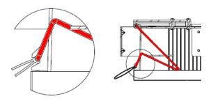
For dismounting, use the strap to disengage the mounting rail. Use a small screwdriver to force the spring away from the rails, and pull the speaker down from the magnets.
